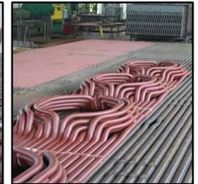
**Job - Description :** Economizer coils, Super heater coils, Re heater coils, Water wall panels
